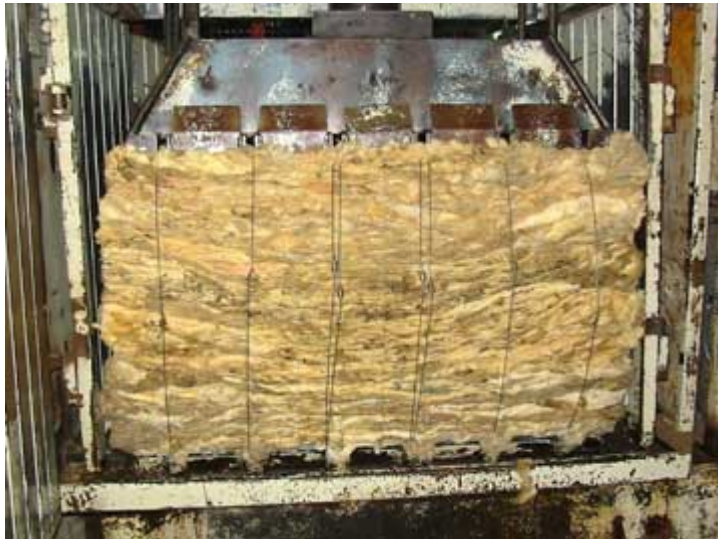
Wired wool bale - cylinder raised for bale removal
