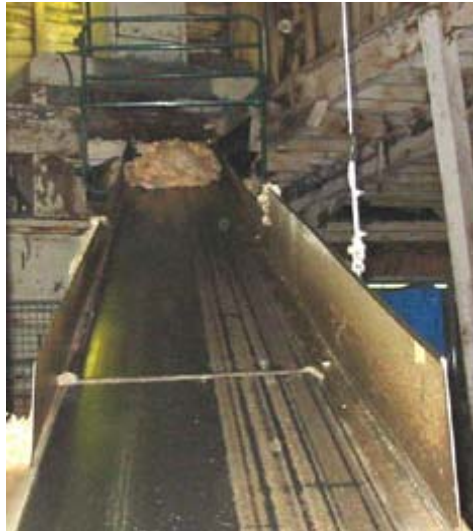
A conveyor feeds the wool press from the wool grading line.
