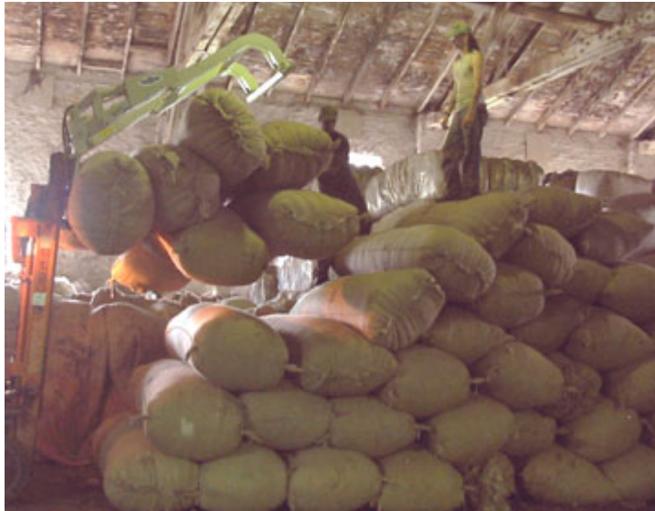
Unloading wool bags with forklift and grapple clamp to storage area until grading
