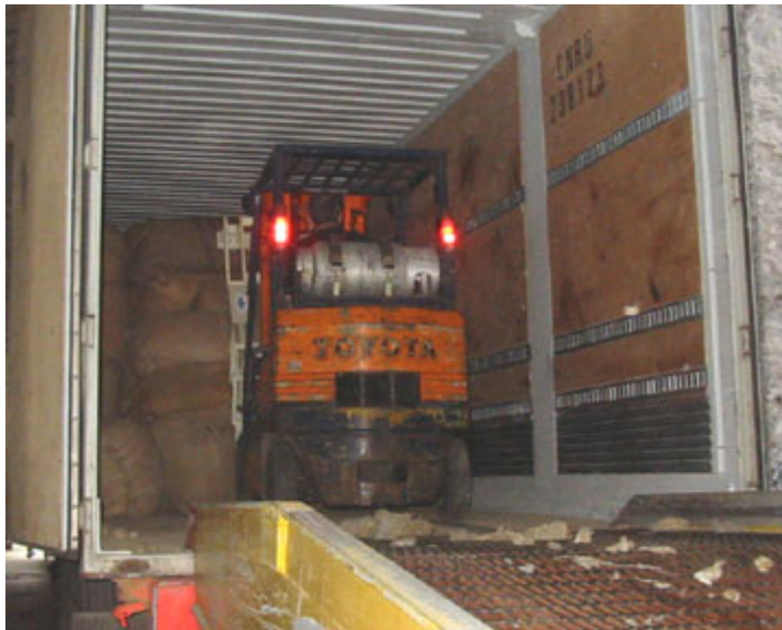
Unloading wool bags from transport truck with modified grapple clamp
