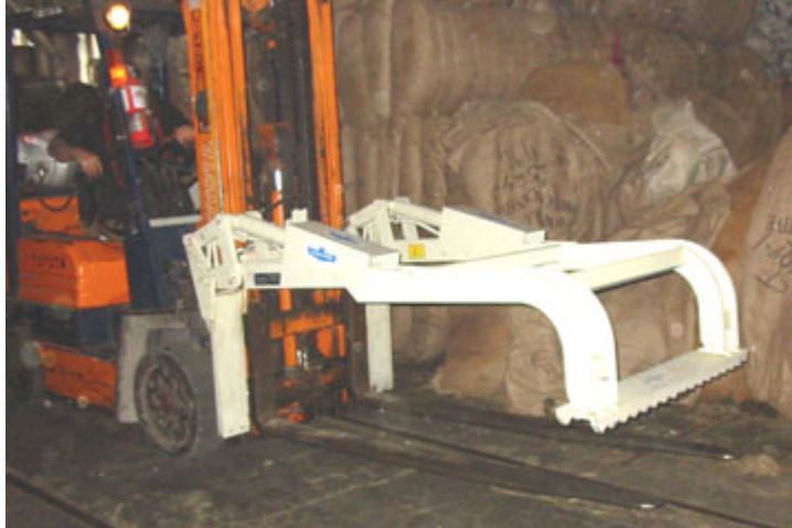
Modified grapple clamp for unloading wool bags at Carleton Place wool grading warehouse.
