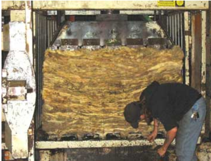
Applying wire ties to compressed wool bale
