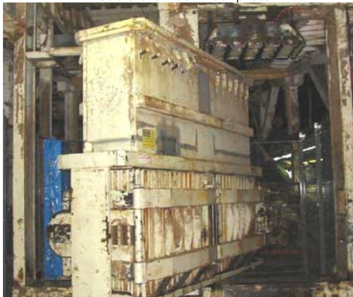
Wool press rotating 360 degrees for final pressing of bale.
